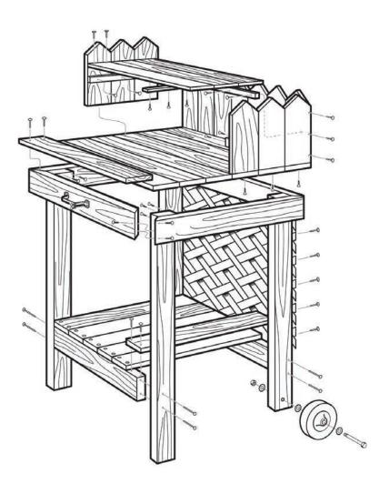
the back cleat along the eight back panel pickets so that it has a 3/4" gap from each end of the back panel sides. The cleat on the back panel should be attached so that the top of the cleat is 5-3/4" from the bottom of the pickets.
